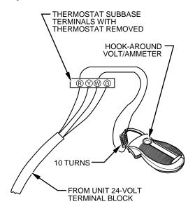
EXAMPLE:  $\frac{5.0 \text{ AMPS ON AMMETER}}{10 \text{ TURNS AROUND JAWS}} = 0.5 \text{ AMPS FOR THERMOSTAT SETTING}$
